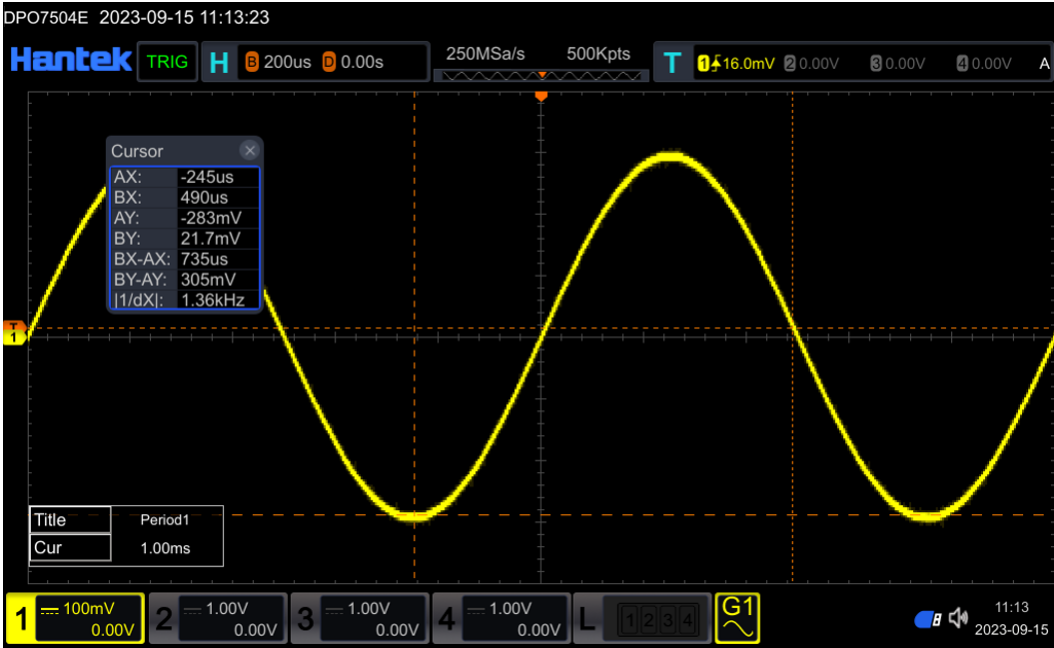
Figure 10.4 Track Measurement (after Horizontal Expansion)
