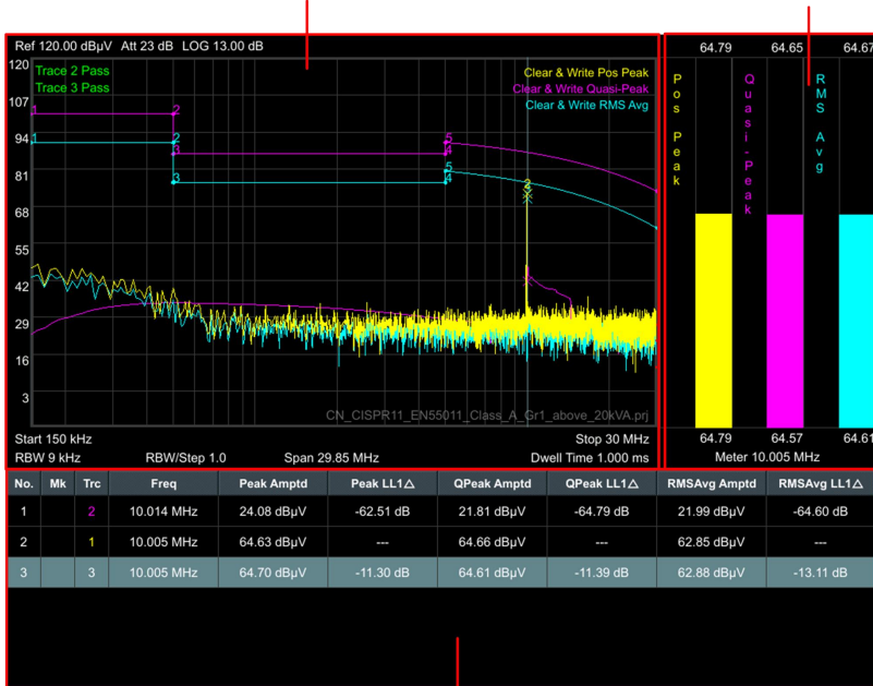
Signal list and its final measurement results are displayed Figure 6-1 EMI measurement interface
